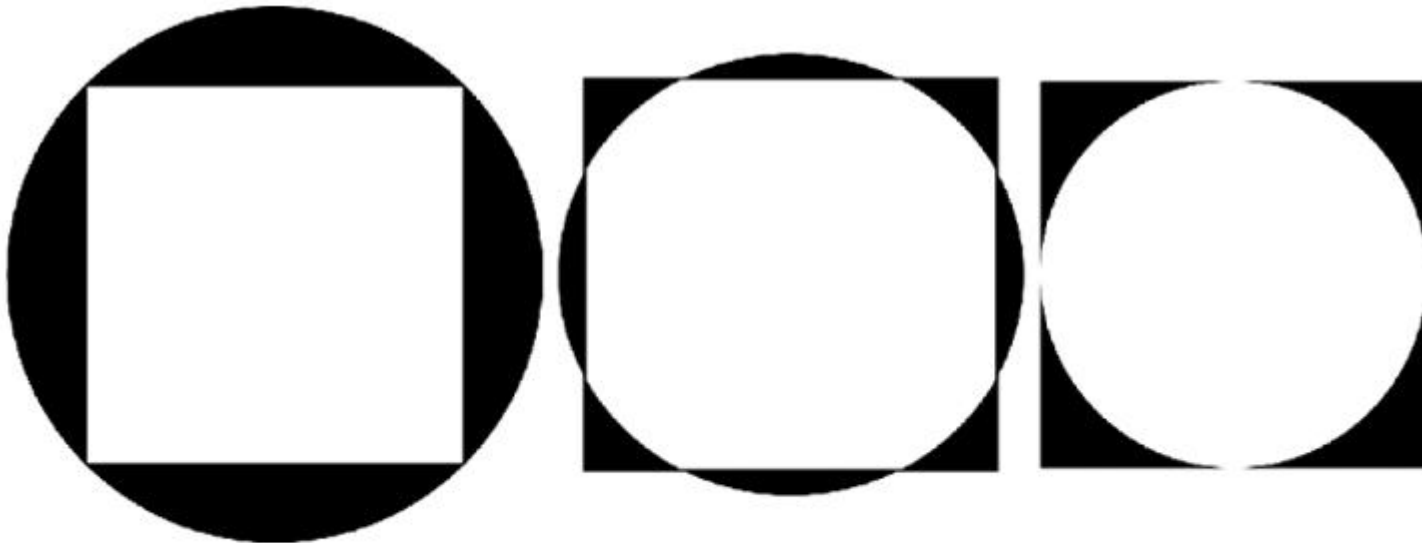
Figure 2.8 Image framing. The focal length of the lens between the image intensifier and the video camera determines the visualized fraction of the output screen. Full overframing is shown on the left, partial in the center, and exact framing on the right. The choice determines the relative use of the image intensifier's physical field of view.
